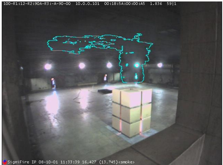
axonX detects smoke in 20 seconds after ignition of a class 2 rack storage fire at the UL large fire test facility in Chicago
